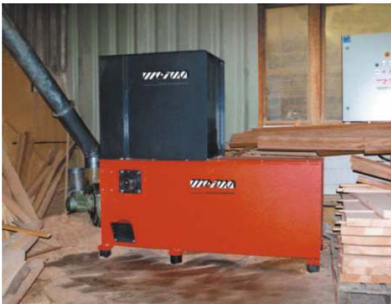
WL 4 S shredder, connected to dust collection system
