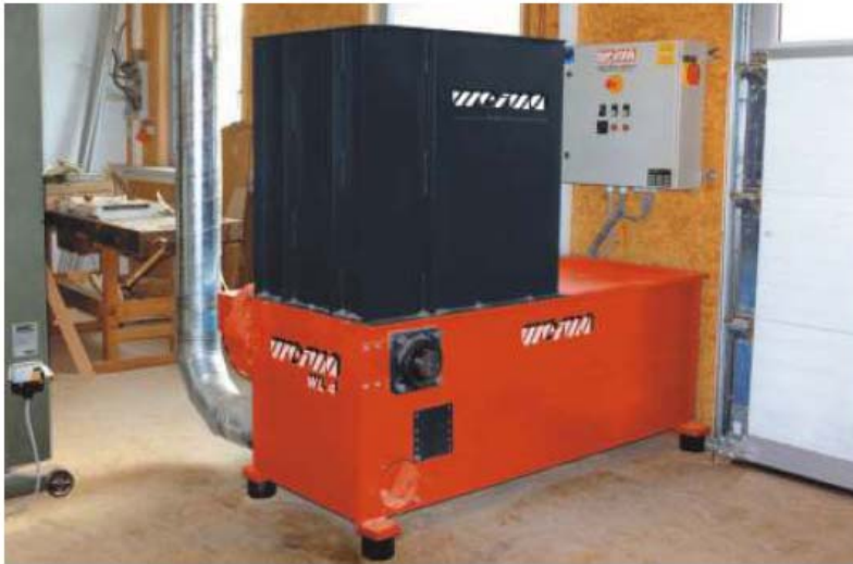
WL 4 shredder, connected to dust collection system
